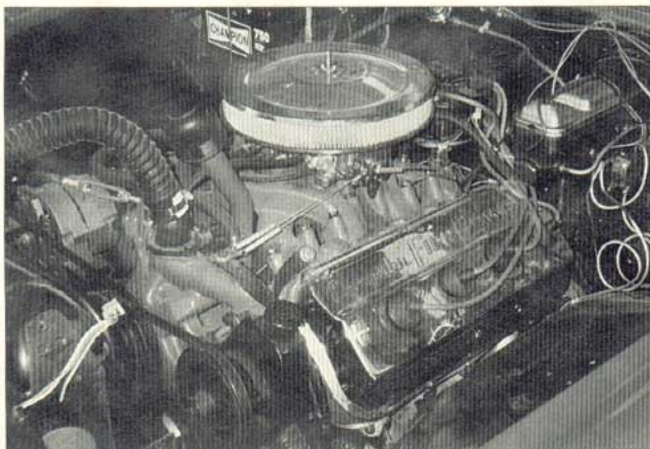
There's nothing like 331 cubes of Chrysler Hemi firepower under the hood. Despite swallowing a piston, the Hemi powered the first C-300 to run in La Carrera Panamericana to the finish. Dual carbs weren't allowed in 1995.
